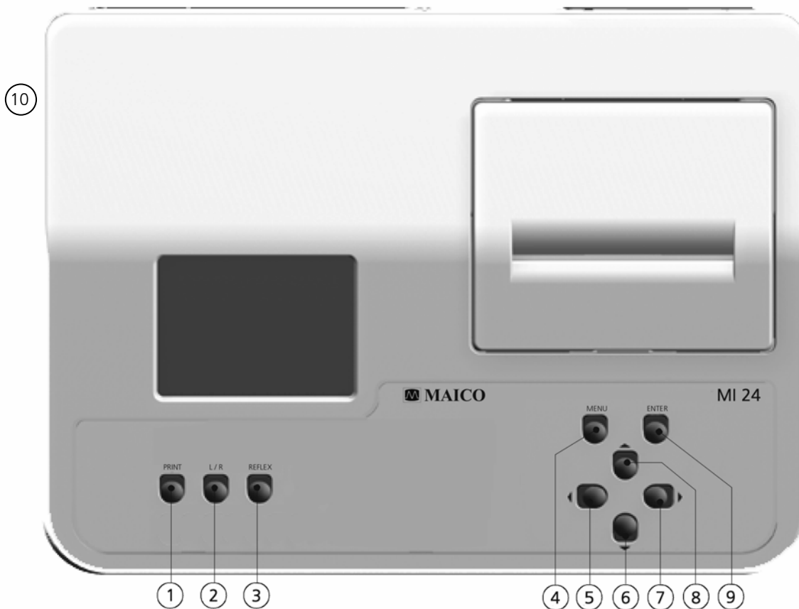
Figure 3 The controls of the MI 24
