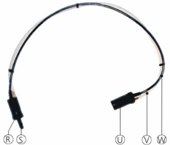
Figure 24 The diagnostic probe insert
